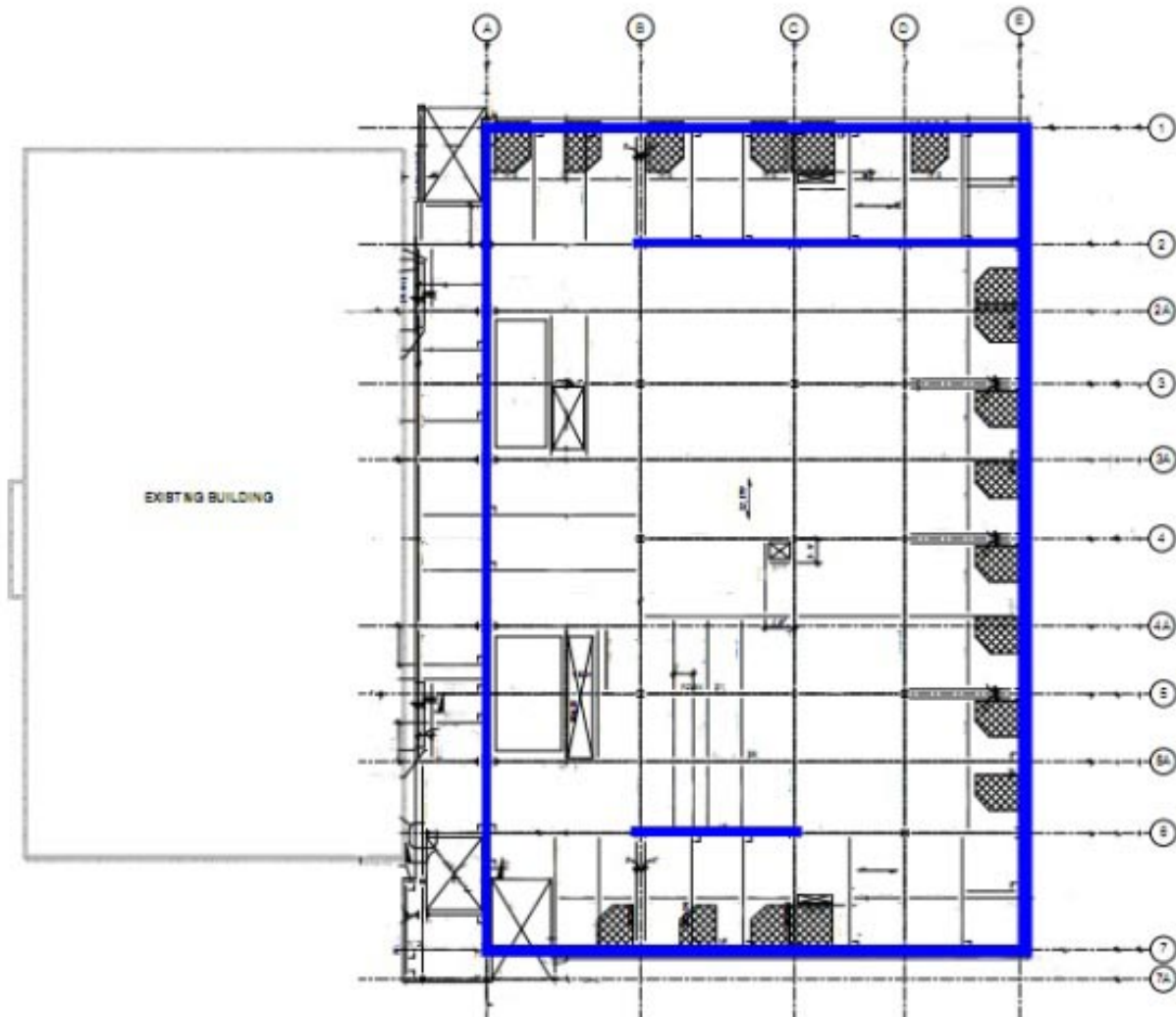
Figure 4: Typical Framing Plans with lateral system highlighted in blue
